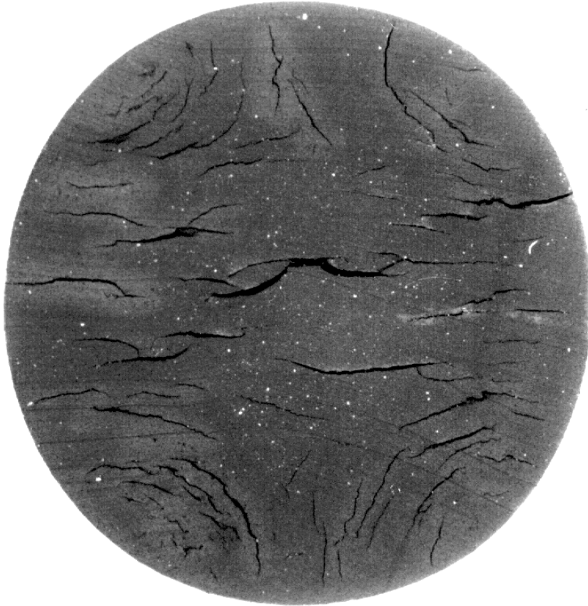
Fig. B.2 - Photograph of typical cross section with RGD damage (Rating # 4) (Reproduced by courtesy of MERL, UK).
